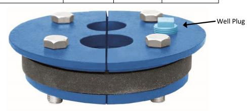
The blue plug in this picture is the well plug/vent. It can be plastic, brass, or galvanized and must be reinstalled. Only use this opening to pour in bleach. Do not loosen the four bolts around the seal or it will impact the ability to prevent contamination. If the plug is made of plastic it can crumble very easily. Best to get a replacement before starting. They can range in size from ¼" to ¾" so measure before purchasing. If in doubt, call a professional.
